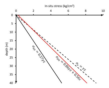
Figure 11. The variation of in-situ horizontal stress  $\sigma_{h0}$  in normall-consolidated deposite soils and  $\sigma_{H0}$  in thrust fault zone.
