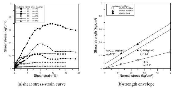
Figure 7. The shear behavior and strengths of faulted mudstone at  $\omega = 10\%$  and 20%.
