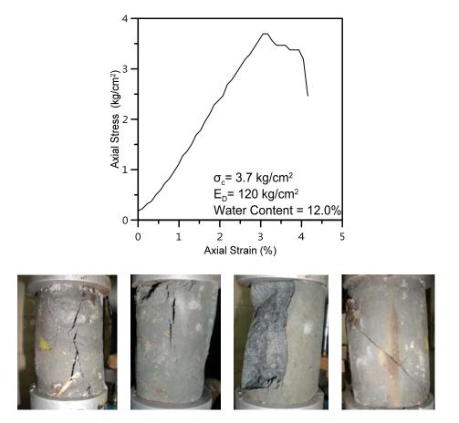
Figure 6. The typical stress-strain behavior of mudstone and fracture mode under compressive test.
