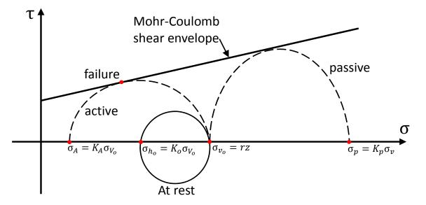
Figure 2. The in-situ horizontal earth pressure decreases from at-rest state to active shear failure due to ground movement.
