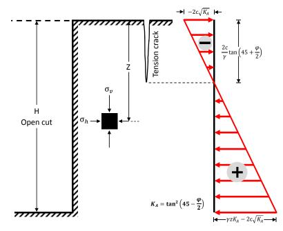
Figure 1. The development of lateral earth pressures and tension crack due to vertical cut.
