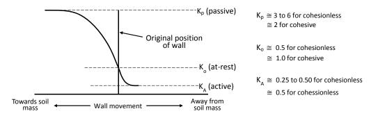
Figure 3. The coefficient of earth pressure decreases from K<sub>0</sub> to K<sub>A</sub> due to ground movement.
