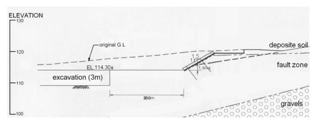
Figure 4. The profile of open cut and previous slope cut in the fault zone.
